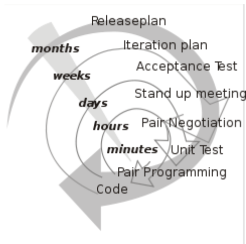
Figure 2-21: Typical time scales associated with elements of the software development life cycle
